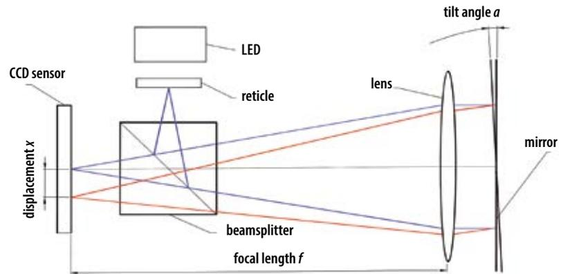
**Fig. 1** Optical schematic illustration of classical autocollimator and telescope into one instrument (Source: Duma Optronics)
