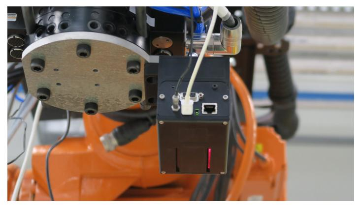
Applications identified for the LAMM sensor include robotic tracking, fixture validation and robotic machining.
