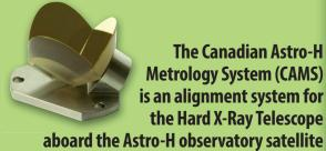
CAMS is designed to measure the lateral/rotational displacement in the spacecraft's optical bench relative to the instruments. PLX designed a 1.94" [49 mm] Invar mounted retroreflector with a 0.5 arc second accuracy, which was used for alignment monitoring.
