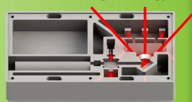
PLX's innovative beam steering technology can achieve equal precision at a low enough cost that one or more scanners can be permanently embedded into manufacturing systems.
