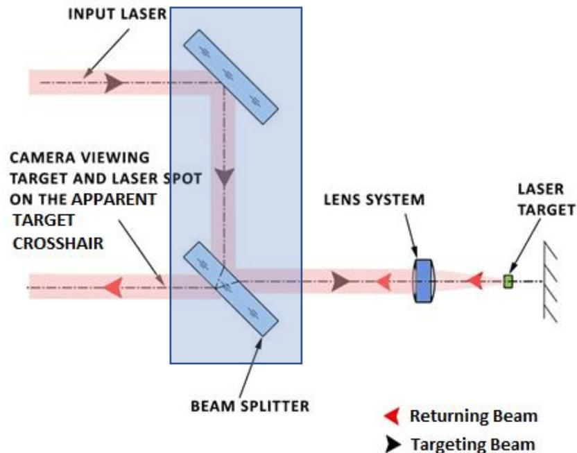
Figure 2 This is a schematic showing a long-range camera, such as an IR camera, which must be perfectly aligned to a laser designator.
