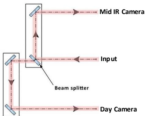
Figure 3 PLX's boresighting system schematic. The input is a collimated multi-wavelength target source. The nightside output goes to a FLIR camera, and the dayside output goes to a high-resolution color camera.
