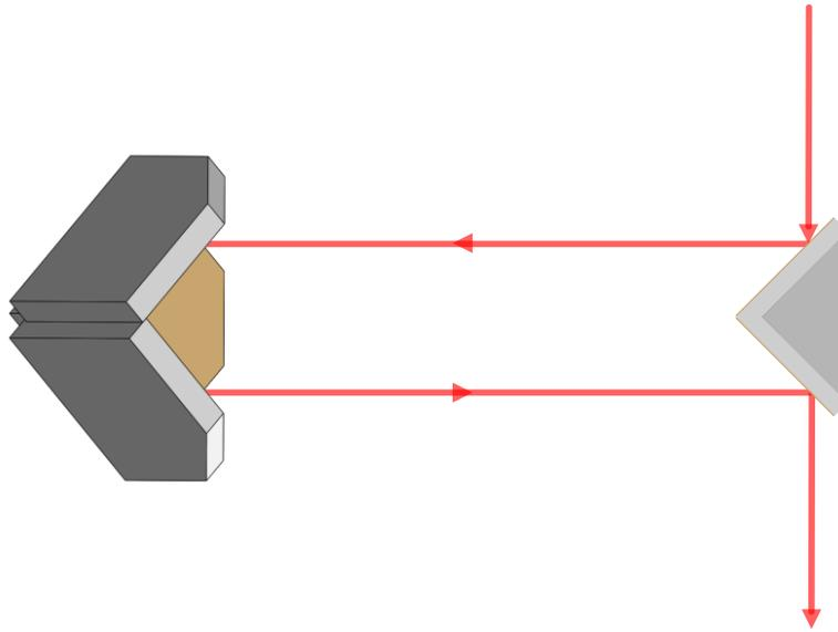
Figure 4 Laser Optical delay line. Figure 4 shows a simple assembly where incoming laser light is reflected by a reverse roof mirror as well as a retroreflector to ultimately return to the original path. This added path provides the delay. The retroreflector can be translated (left to right in the figure) to vary the optical delay, without affecting the optical alignment of the system.
