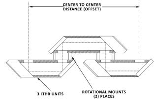
A THREE LTHR COMBINATION FOR LONG DISTANCE ALIGNMENT. THE ROTATIONAL MOUNT ENABLES ALIGNMENT FOR AN ADDITIONAL AXIS.
