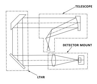
SETUP FOR DETECTOR MOUNT ALIGNMENT
