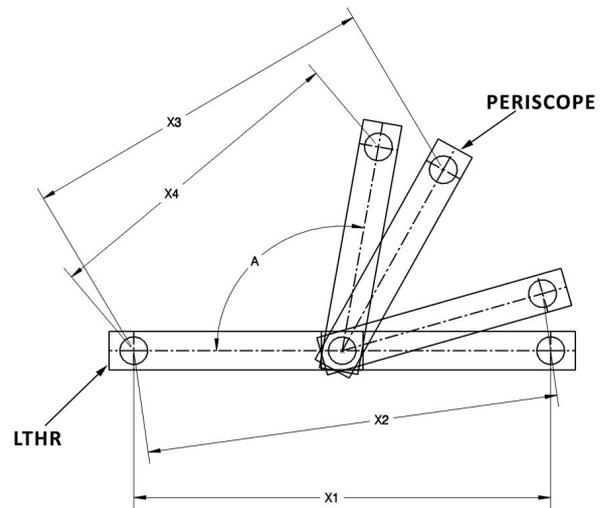
MULTIPLE CONFIGURATION DISTANCE "X" AS A FUNCTION OF ANGLE "A"
