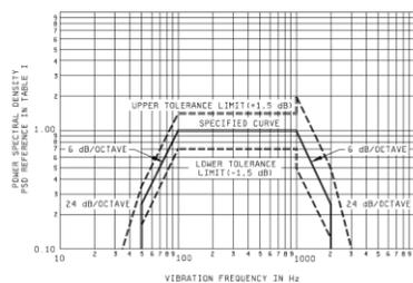
FIGURE 2026-1 Test condition I random vibration test curve envelope (see table 1)
