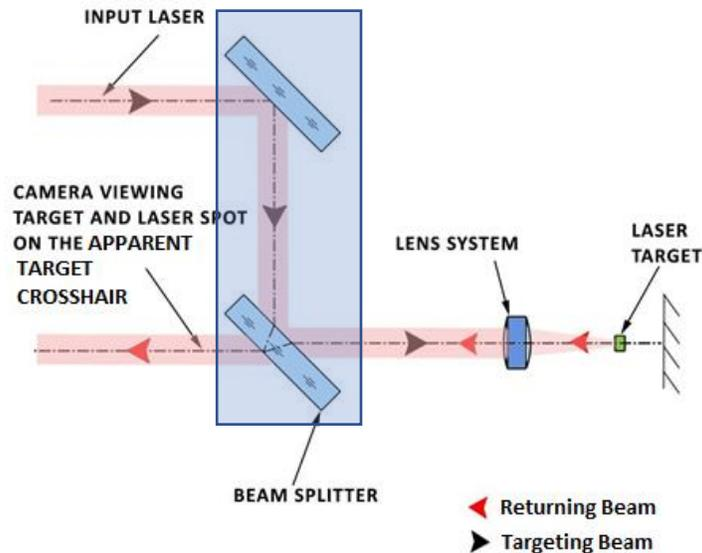
Figure 5 This is a schematic showing a long-range camera, such as an IR camera, which must be perfectly aligned to a laser designator.
