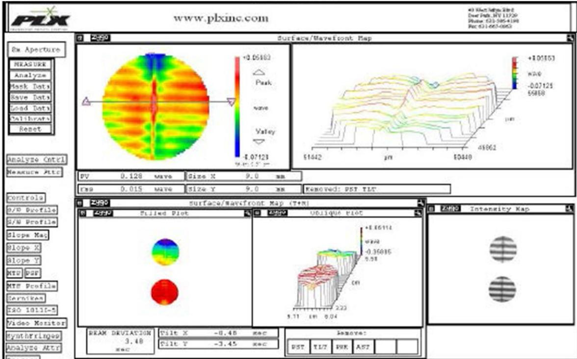
Figure 4 ZYGO testing result of a M.O.S.T unit
