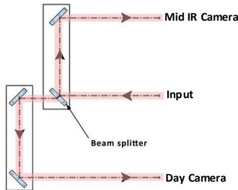
Figure 7 PLX's bore sighting system schematic. The input is a collimated multi-wavelength target source. The nightside output goes to a FLIR camera, and the dayside output goes to a high-resolution color camera.
