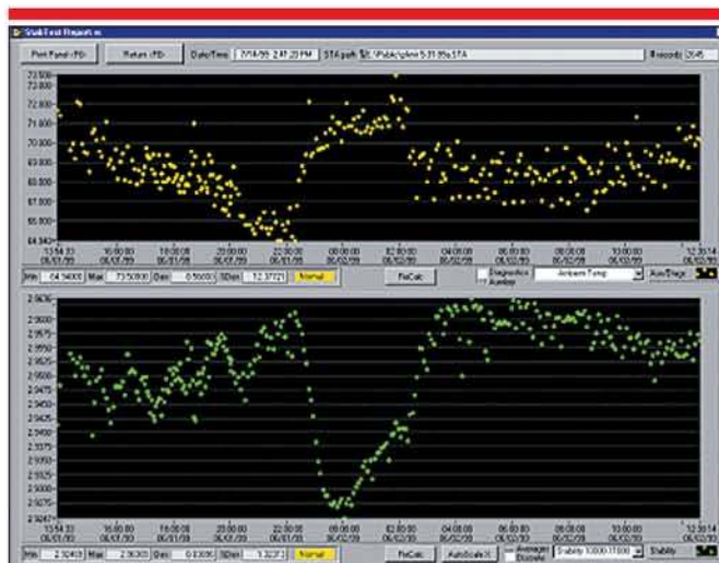
Figure 8. Stability test data from the interferometer.
