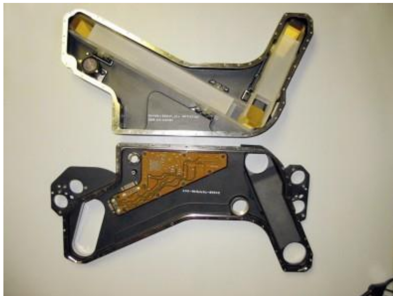
Figure 8. Image of the actual Boresighting system unit, with the two halves of the housing opened to show the two LTHR™ assemblies.
