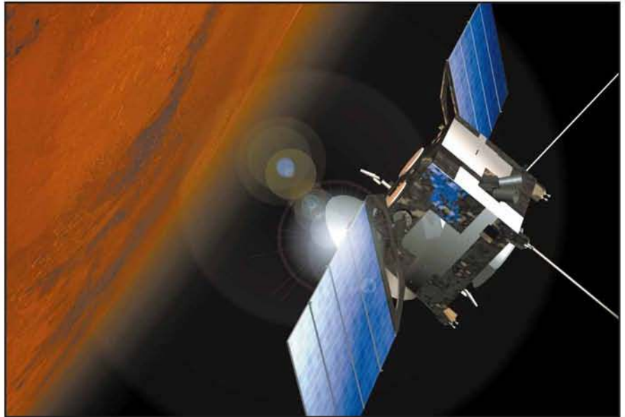
The European Space Agency's Mars Express will investigate the red planet from orbit and from the surface. The craft's orbiter features the Planetary Fourier Spectrometer, which employs novel hollow retroreflectors.
