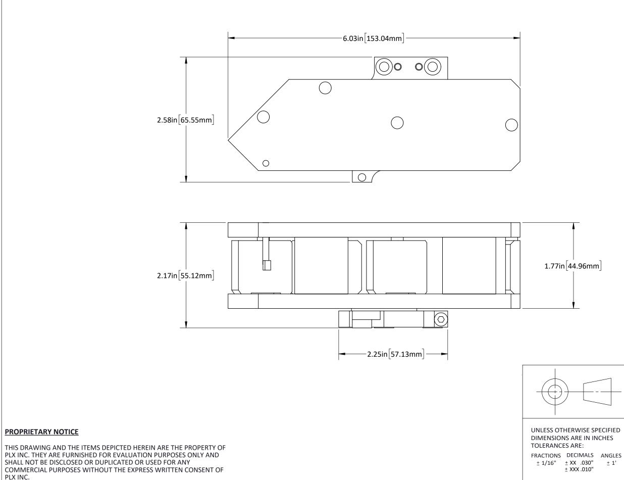
INNOVATIVE OPTICAL SYSTEMS Ø 1.00" NIR Monolithic Michelson Interferometer Assembly INT10-M ± XXX .010"
