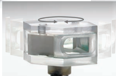
▶ Monolithic scanning device Designed to oscillate at a rate higher than 1KHz, while maintaining its stability and accuracy, this lightweight structure is balanced to reduce the moment of inertia about the pin axes.
