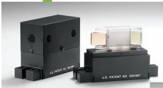
▶ Monolithic scanning device Designed to oscillate at a rate higher than 1KHz, while maintaining its stability and accuracy, this lightweight structure is balanced to reduce the moment of inertia about the pin axes.
